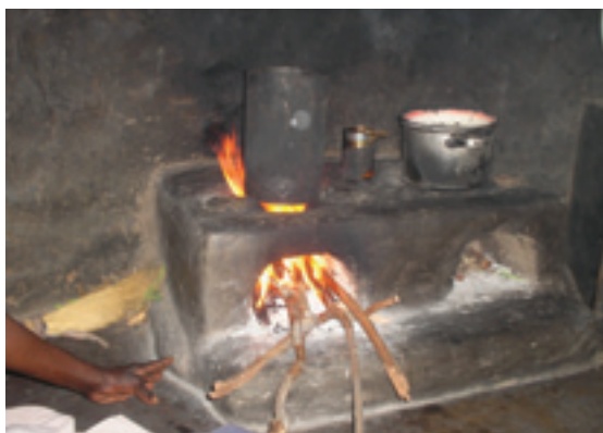
Figure 3 A twin upesi stove installed in a kitchen in Kenya
